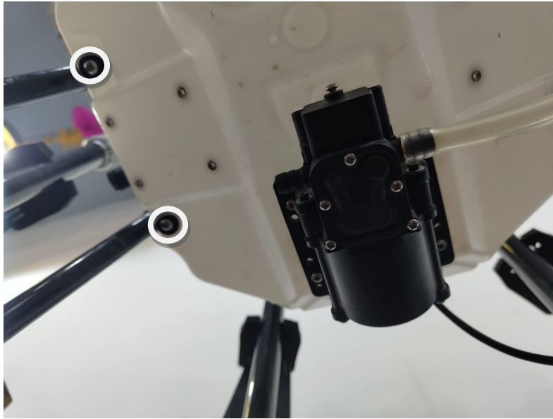
Figure 6: M5 Allen bolt to hold the tank, ensure tightness of the bolts after every 50 flights
