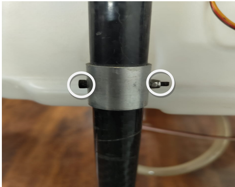
Figure 8: M3 Allen bolt and nut to hold the clamp holding the tank, Ensure tightness at all 4 sides after every 50 flights
