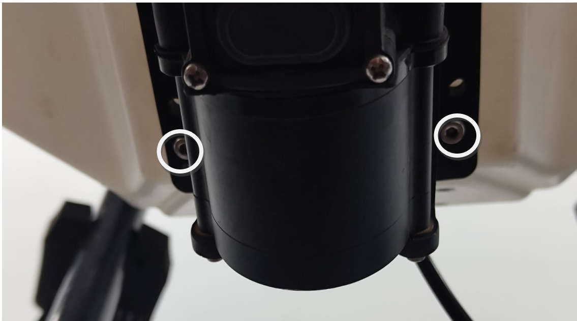
Figure 9 M3 Allen bolts to hold the pump, ensure tightness after every 50 flights
