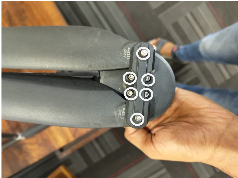
Figure 5: M3 propeller mount bolts, tightness to be ensured after every 2 flights
