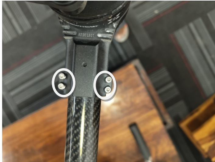
Figure 4: M3 Allen bolts for motor mounting, tightness to be ensured after every 100 flights
