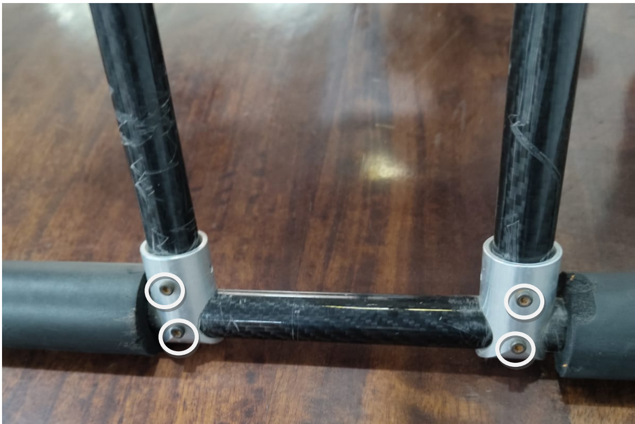
Figure 11 M3 bolts to hold the landing gear , ensure tightness after every 50 flights
